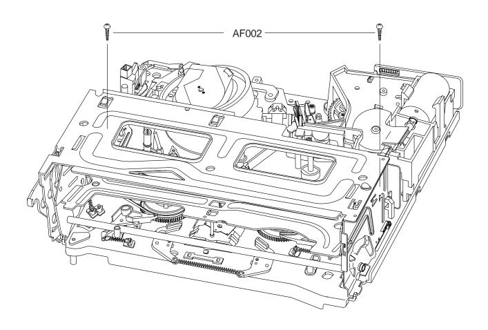
Fig.3-1 FRONT LOADING ASS'Y SEPARATION
